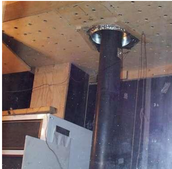
Figure 1. The air conditioner was arranged to discharge into a perforated false ceiling to reduce air turbulence in the test enclosure. The white box is the air conditioner and the plywood box above it is the discharge duct leading to the plenum above the perforated ceiling.
